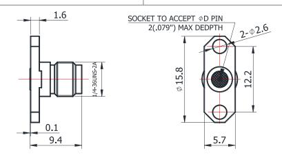
For glass-bead of 0.46mm pin diameter
