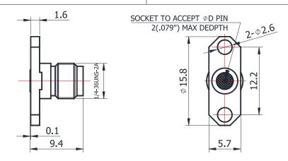
For glass-bead of 0.38mm pin diameter
