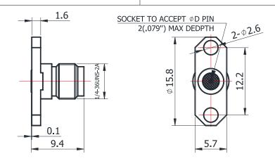
For glass-bead of 0.30mm pin diameter
