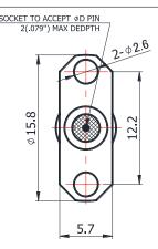
For glass-bead of 0.23mm pin diameter
