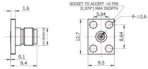
For glass-bead of 0.51mm pin diameter
