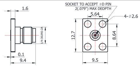
For glass-bead of 0.46mm pin diameter
