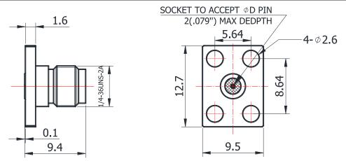
For glass-bead of 0.30mm pin diameter
