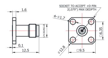
For glass-bead of 0.30mm pin diameter
