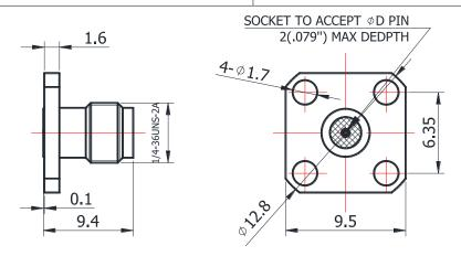
For glass-bead of 0.23mm pin diameter
