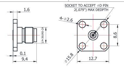
For glass-bead of 0.46mm pin diameter
