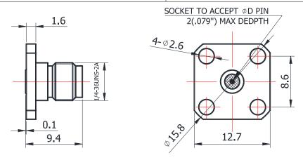
For glass-bead of 0.30mm pin diameter
