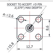
For glass-bead of 0.23mm pin diameter
