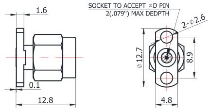
For glass-bead of 0.46mm pin diameter
