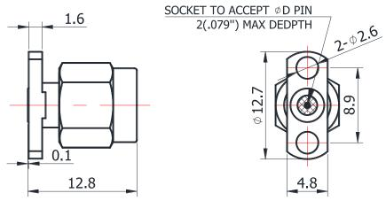
For glass-bead of 0.38mm pin diameter
