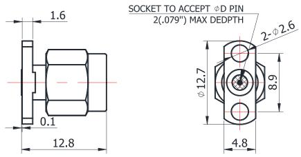
For glass-bead of 0.23mm pin diameter
