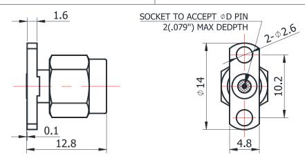
For glass-bead of 0.51mm pin diameter
