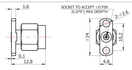
For glass-bead of 0.30mm pin diameter
