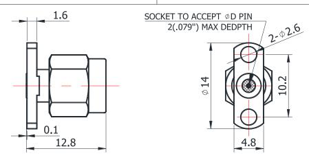
For glass-bead of 0.23mm pin diameter
