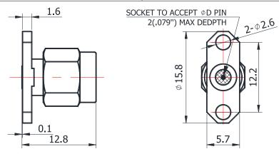
For glass-bead of 0.51mm pin diameter
