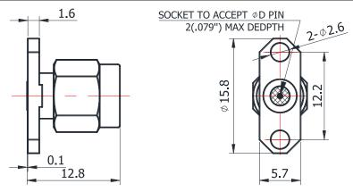
For glass-bead of 0.46mm pin diameter
