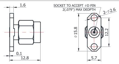
For glass-bead of 0.30mm pin diameter
