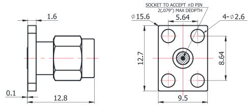
For glass-bead of 0.38mm pin diameter
