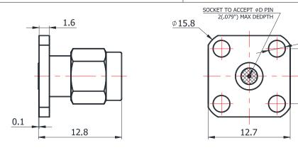
For glass-bead of 0.46mm pin diameter
