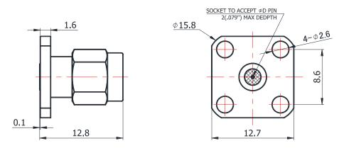
For glass-bead of 0.38mm pin diameter
