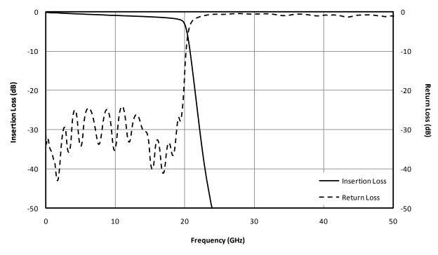
Fig. 1. Magnitude response for a typical FLP-2000.
