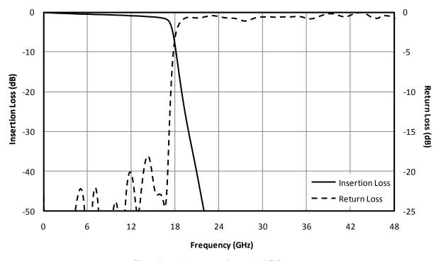
Fig. 1. Magnitude response for a typical FLP-1740.
