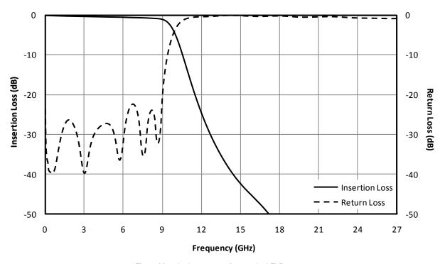
Fig. 1. Magnitude response for a typical FLP-0960.
