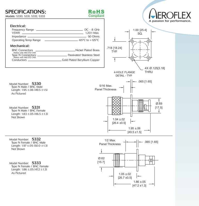
Note: Dimensions in Brackets are Expressed in Millimeters and are for Reference Only.
