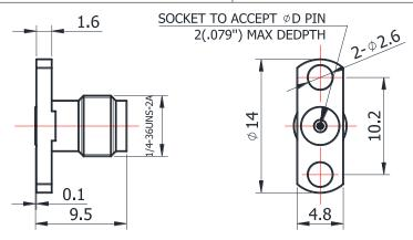
For glass-bead of 0.51mm pin diameter
