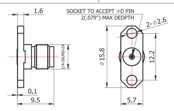
For glass-bead of 0.30mm pin diameter
