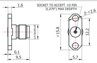
For glass-bead of 0.23mm pin diameter
