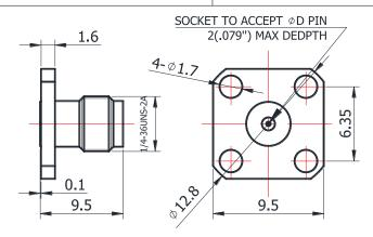
For glass-bead of 0.30mm pin diameter
