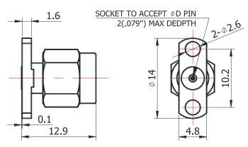
For glass-bead of 0.38mm pin diameter
