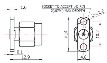
For glass-bead of 0.30mm pin diameter
