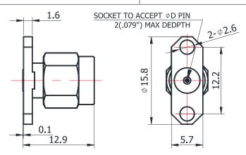
For glass-bead of 0.30mm pin diameter
