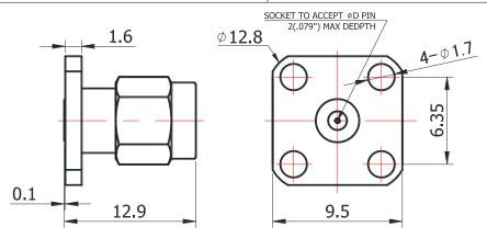
For glass-bead of 0.38mm pin diameter
