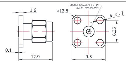
For glass-bead of 0.30mm pin diameter
