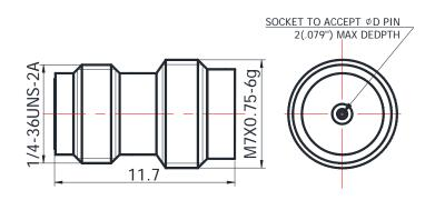
For glass-bead of 0.30mm pin diameter
