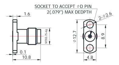
For glass-bead of 0.51mm pin diameter
