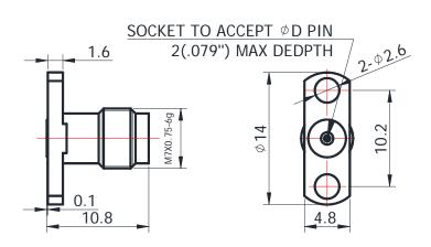
For glass-bead of 0.30mm pin diameter
