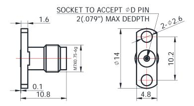
For glass-bead of 0.23mm pin diameter
