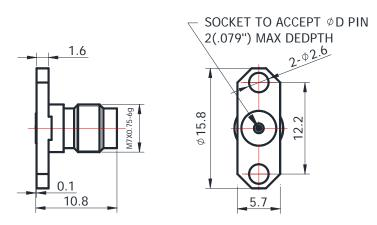
For glass-bead of 0.51mm pin diameter
