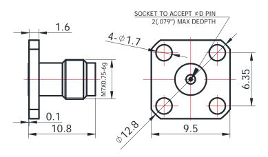
For glass-bead of 0.51mm pin diameter
