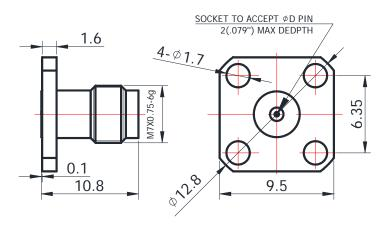
For glass-bead of 0.30mm pin diameter
