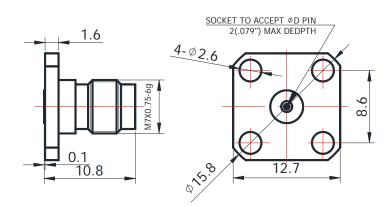
For glass-bead of 0.51mm pin diameter
