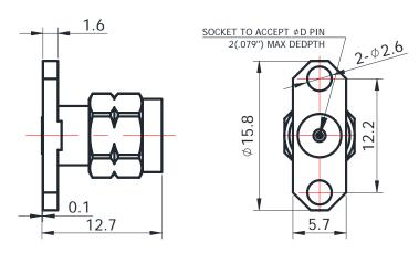
For glass-bead of 0.23mm pin diameter
