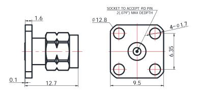
For glass-bead of 0.30mm pin diameter
