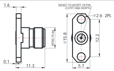
For glass-bead of 0.23mm pin diameter
