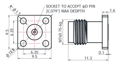
For glassbead of 0.30mm pin diameter
