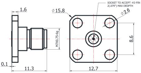
For glass-bead of 0.23mm pin diameter
